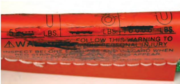
THE DAMAGE: Knots compromise the strength of all slings by not allowing all fibers to contribute to the lift as designed.
