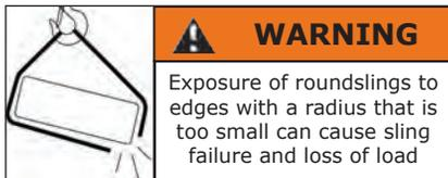
Edges do not need to be “sharp” to cause failure of the sling. The following table shows the minimum allowable edge radii suitable for contact with unprotected roundslings. Chamfering or cutting off edges is not an acceptable substitute for fully rounding the edges to the minimum radius. Slings can also be damaged from contact with edges or burrs at the sling connection.
