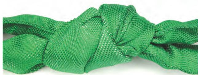
THE DAMAGE: Cuts to the cover NOT exposing internal core yarns –*Tuflex* roundslings all have a double walled jacket protecting the inner core yarns from damage. If damage (except for chemical or heat) appears only to the outer jacket and does not expose the inner core yarns, the sling may remain in service. To extend sling life, the sling may be returned to Lift-All for inspection and application of a patch to cover the damaged area.
